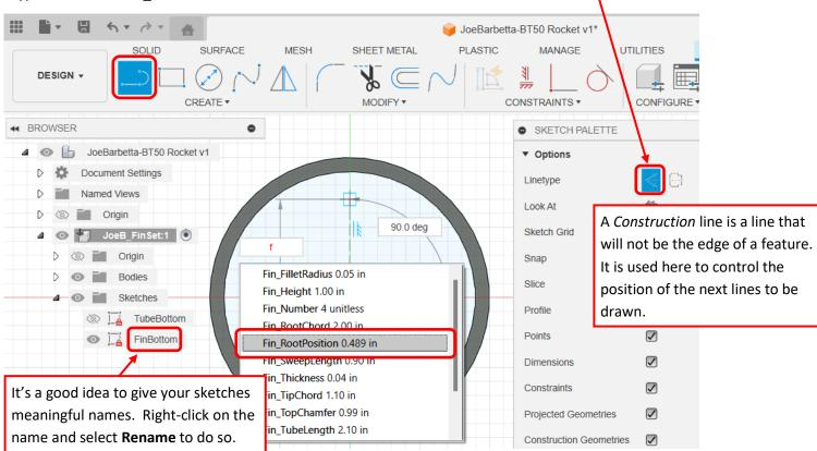
This is what that line should look like. The dash pattern of the line indicates it is a Construction line. It is OK if the thin black dimension lines look different.
