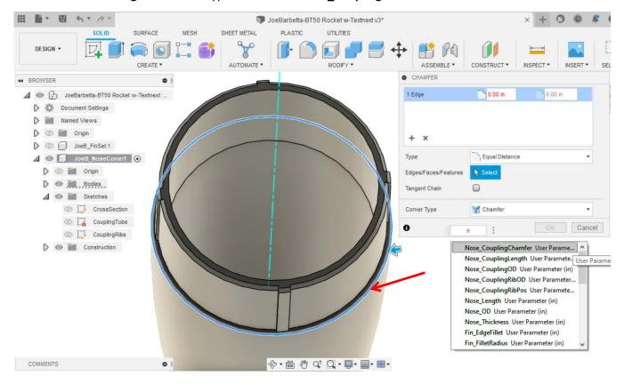
This is now how the side view looks. Note the 45 degree chamfer.
