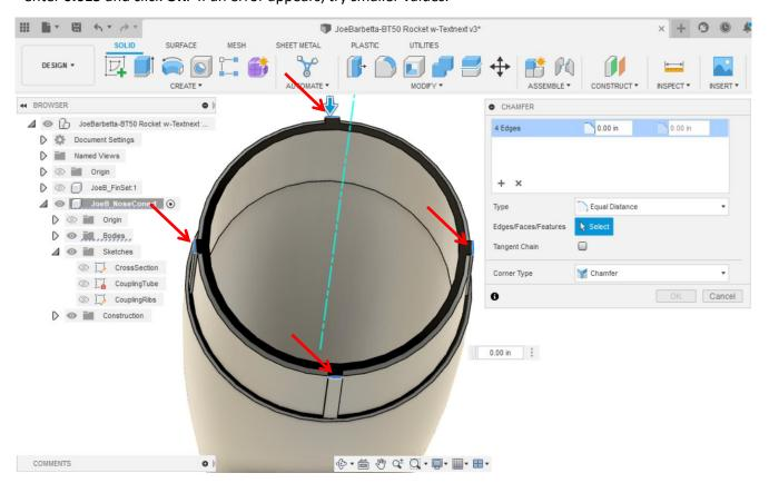
Because the nose cone will be printed when flipped 180 degrees compared to below it will start printing from what is now the top surface. When the print reaches the layer where the coupling tube meets the nose cone it will encounter an overhang. Adding a chamfer will allow adherence to the 45 degree rule.
