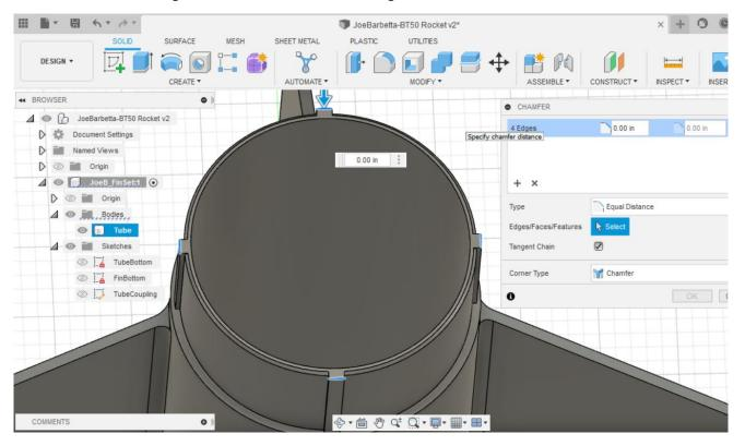
The coupling section has a thin wall thickness that should be made thicker. This is an opportunity to change a parameter.
