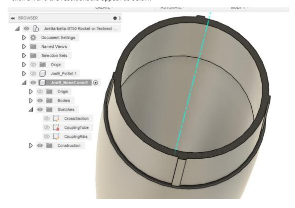
Now some chamfers will be added to make it easier to insert the nose cone in the body tube.
