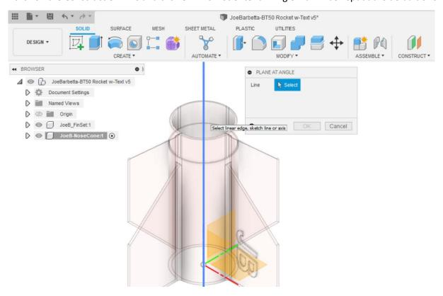
Here the view was changed to show this new vertical plane through the center of the Fin Set. One needs to create a *Construction Plane* if needed for a new sketch that can't be started on an existing plane or object face.
