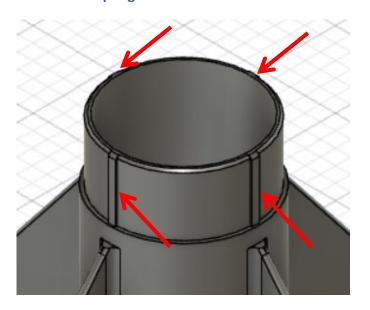
**3D** printed parts do not always print accurately. For example, the inner and outer dimensions of a tube can vary about 0.01". This tolerance doesn't matter for many dimensions, however, when components must fit together this can be a problem.
