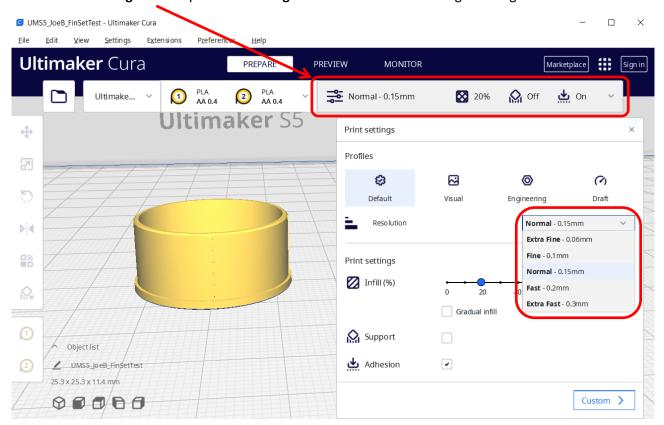
The Resolution setting is a compromise between quality and print speed. A thinner layer will result in better accuracy for top surface features. For example, the top of any angled or rounded surfaces will appear smoother with smaller resolutions because each layer is thinner. When prioritizing printing speed, a larger resolution for thicker layers can be selected.
