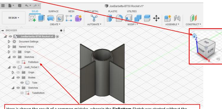
Here is shown the result of a common mistake, wherein the **FinBottom** *Sketch* was started without the **JoeB\_FinSet** being the *Active Component*. If this occurred, **right-click on the** *Sketch* **name and select Activate** and then **drag the** *Sketch* **name onto the FinSet** *Component* **name**, e.g. JoeB FinSet here.
