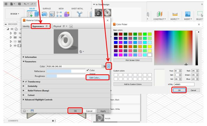
If there are components in a project, wherein different colors are desired, the white ABS plastic icon in the Plastic folder can be used again and then the new white icon in the top section can be edited to a different color.
