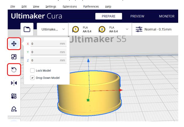
If an object is opened and is not in the proper orientation, the Rotate tool can be selected and the rotate arrows for the desired axis can be clicked on and moved. The angle will jump in 15 degree increments to make it easy to rotate an object.
